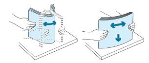
For transparencies; hold the transparencies by the edges and avoid touching the print side. Oils from your fingers that are deposited on the transparency can cause print quality problems. If you are using the transparencies with paper backing, insert a sheet of plaing paper on the tray before loading transparencies. Doing so prevents paper jams while feeding.
